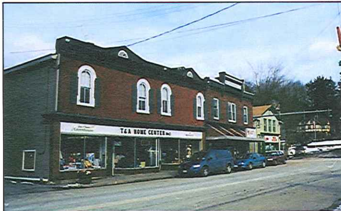
Above: Notice the pitched or sloped rooflines in each of these buildings which are concealed behind a parapet wall that also incorporates a decorative upper cornice.
